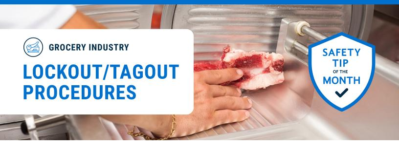
Machines can become energized unexpectedly during maintenance and cleaning, resulting in serious or fatal injury. A lockout/tagout program and compliance with OSHA's lockout/tagout standard can prevent incidents.
